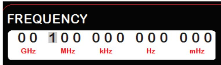
To change any setting, click on a digit in the appropriate window and the number will be highlighted (figure above). Enter the desired value and press return on the PC keyboard. Other digits can be modified by using the mouse, or the right and left arrow keys.
