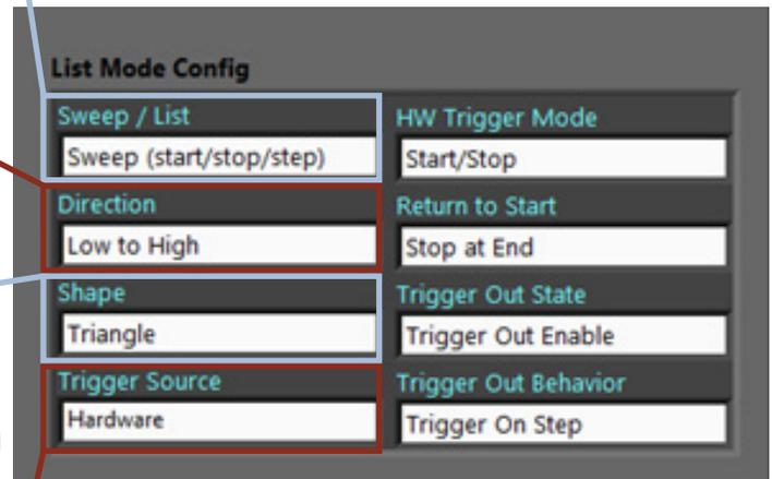
6.4 Trigger Source can be changed to **Hardware** or **Software**.
