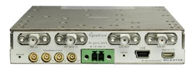
any external signal source capable of tuning over the range of the SC5313A (like the SignalCore SC5506A dual channel signal source). The SC5313A can daisy-chain the LO signal, allowing a single source module to drive multiple direct IQ downconverters for coherent reception.
