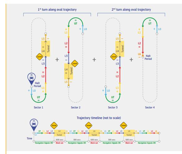
FIGURE 6: SKETCH OF A POSSIBLE OPEN SKY VEHICLE TRAJECTORY TO BE USED IN THE DYNAMIC SCENARIO SPECIFED IN SECTION 2.2.4 OF ANNEX VI [1], INCLUDING THREE INTERVALS WITH A COMPLETE OUTAGE OF NAVIGATION SIGNALS, AND THE ASSOCIATED TIMELINE INDICATING THE TIME SERIES OF ALL THE TRAJECTORY SECTORS INVOLVED; © GSA/JRC
