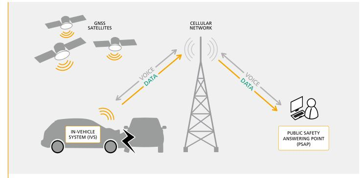
FIGURE 2: FUNCTIONALITY OF ECALL UNITS.
