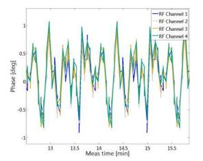
FIGURE 3: PHASE DRIFT OVER MULTIPLE RF OUTPUTS
