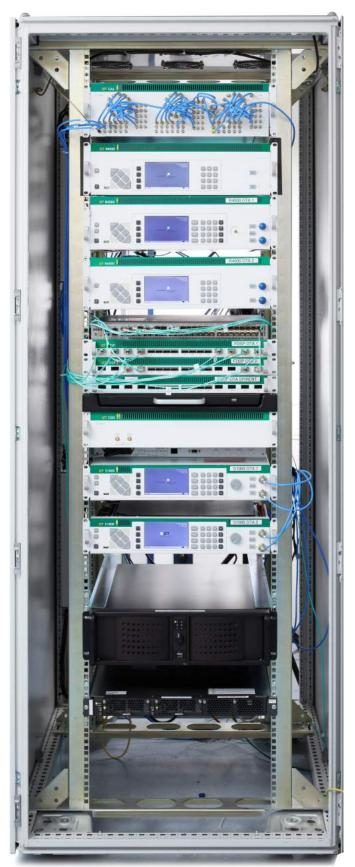
The IZT C7000 is a high-performance MIMO Simulator for the frequency range of 30 MHz to 6000 MHz with 80 MHz instantaneous bandwidth. The very low and adjustable input to output latency enables efficient testing of modern communciation systems. The digitized signals are sent to the FPGA processor via optical cables to avoid loss of performance due to coaxial cables.
