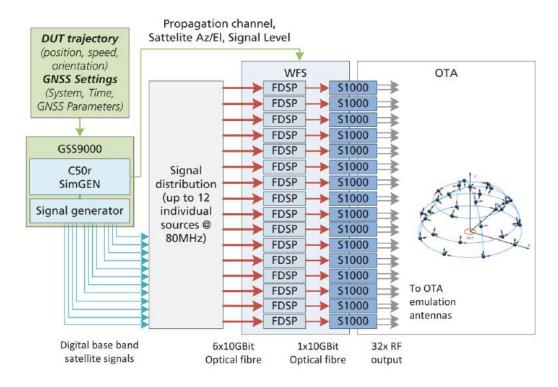
FIGURE 13: CUSTOMER INSTALLATION OF GNSS OVER WFS
