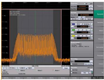
FIGURE 4: FM MODULATION AND OCCUPANCY MEASUREMENT
