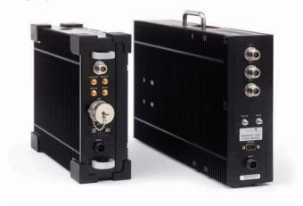
The compact variant of the sucessfull R3000 series combines a limited weight of under 7 kg with a fanless design suited for harsh environments while maintaining the excellent HF performance and a real-time bandwidth of 24 MHz.
