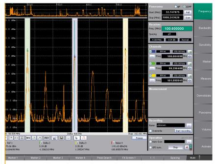
FIGURE 2: PANORAMA SCAN AND 4 MHZ SPECTRUM DISPLAY WITH THREE ACTIVE DEMODULATION CHANNELS
