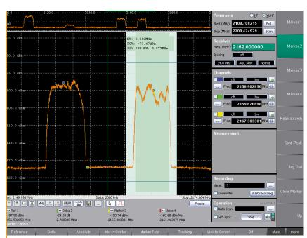
FIGURE 3: PANORAMA SCAN AND BANDWIDTH MEASUREMENT OF OFDM SIGNAL
