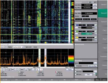
FIGURE 1: COMBINED SPECTRUM AND WATERFALL DISPLAY
